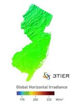
**Solar Resources**- New Jersey has a moderate solar resource, good for residential and commercial electricity generation and non-electric solar thermal generation.
