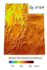
**Solar Resources-** The state's potential for electricity generation provided by solar resources is 69 million MWh per year (NREL).
