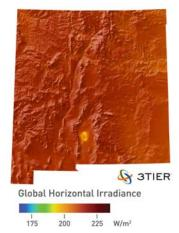
**Solar Resources-** Dark red indicates the highest potential. New Mexico has enough solar resources to produce 6.5 kWh to 7 kWh per square meter, totaling 104 million MWh per year.
