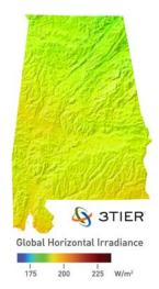
**Solar Resources-** Alabama receives between 185 and 200 W/m<sup>2</sup> of solar radiation, a moderate solar resource potential.
